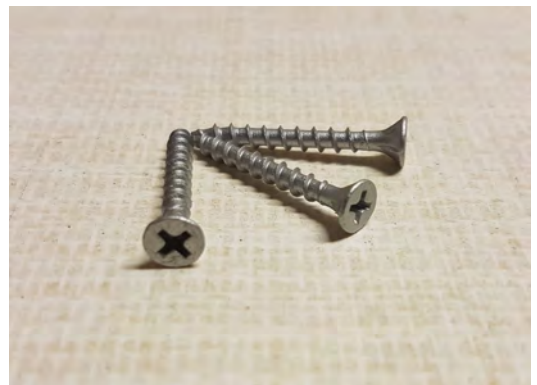
Fortress Fasteners 6g x 32mm C3 Galvanised Collated Screws loose for fixing Magnum Board to timber framing
