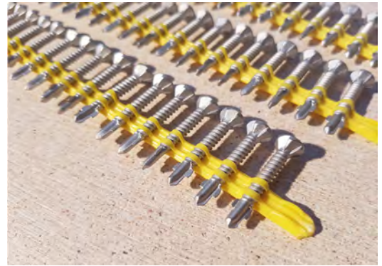
Simson Strong Tie 6g x 32mm C3 Galvanised Collated Square Drive Screws for fixing Magnum Board to steel framing
